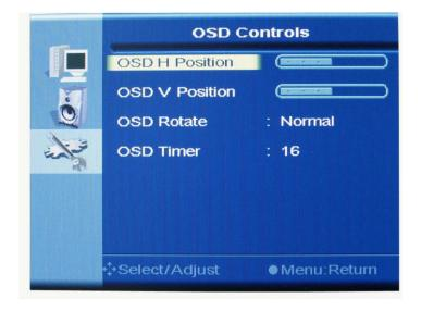
b. Press " " or " " to adjust the horizontal position of OSD menu. Then press "1" to confirm the adjustment and back to OSD Controls sub-menu.
